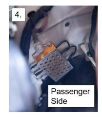
5. Plug in the connector pictured to the OEM fog light connector and leave the 2-pin weather pack out ready to receive the Squadron connector.
