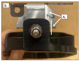
10. Install the Squadron to both metal bracket's lower holes. Use a 4mm Hex key to install a small M6 Button head (B1) and a long M6 Button head. The longer M6 buttonhead (B2) will require the use of the spacer provided and will go onto the larger metal bracket. Adjust the light until it is straight and tighten the bolts.
