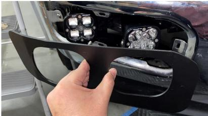
**Step 10:** Observe the angles of the lights. If they need to be adjusted remove the fascia and adjust their height or their angle. Otherwise, fully tighten down the M5 nylocs in the rear (E). Repeat steps 2-10 for the opposite side.
