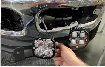
**Step 6:** Loosely install your main bracket inside the fog pocket using 1X M5 Button head and M5 washer (C) and a 2.5 mm Hex tool. Adjust the lights to your preference.
