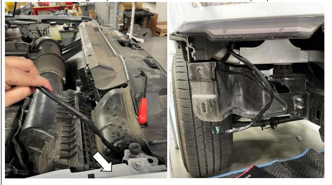
**Upfitter Only** Locate and detach the upfitter fuse box located near the PS fuse box (boxed) by pressing in the two locking tabs (1&2) and lifting up to access the bundle of wires underneath it. Take the included upfitter wiring harness and attach the white wire scotchlok (I) to the desired auxiliary wire using a set of pliers. Reinstall the upfitter fuse box. Attach the connector on the upfitter harness to the harness end (F).
