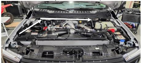
Locate the white connector (K) that attaches the switch to the main harness and disconnect it. With a pick, remove the wire terminals from the connector. Run the switch lead, terminals first, through the wire passthrough (circled) starting inside the cab. Pull the cable through once you are past the grommet and up to your main harness. Reinstall the terminals into the connector and reattach it to the main harness.
