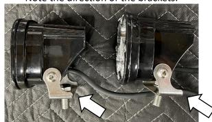
**Step 5:** Install your lights onto the provided brackets as shown using a 9/16" wrench and socket. The light face should be parallel to the edges (B) outlined below. **Note: SAE's must be placed on the outer positions. Lights with a Spot lens equipped (Excluding SAE) should be equipped on the inner location.**
