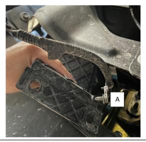
**Step 3:** Remove the Fog pocket plastic trim piece by squeezing the tabs from behind and pushing outward.
