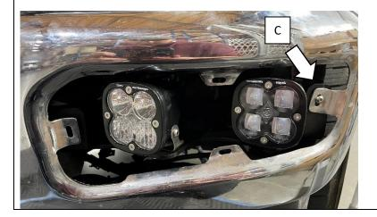
**Step 7:**Cut a 10in section from your EPDM. Cut this strip horizontally so that you have two thin 10" sections. Cut a 4.25" section from your EPDM. Install the EPDM onto your bracket as shown lining up the straight edges as shown. Trim to match the bracket shape as seen on the dotted lines.
