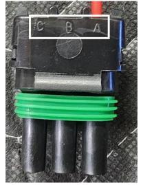
Using the table below, press the wires into their designated location. Once all wires are locked in place, close the clamshell.
